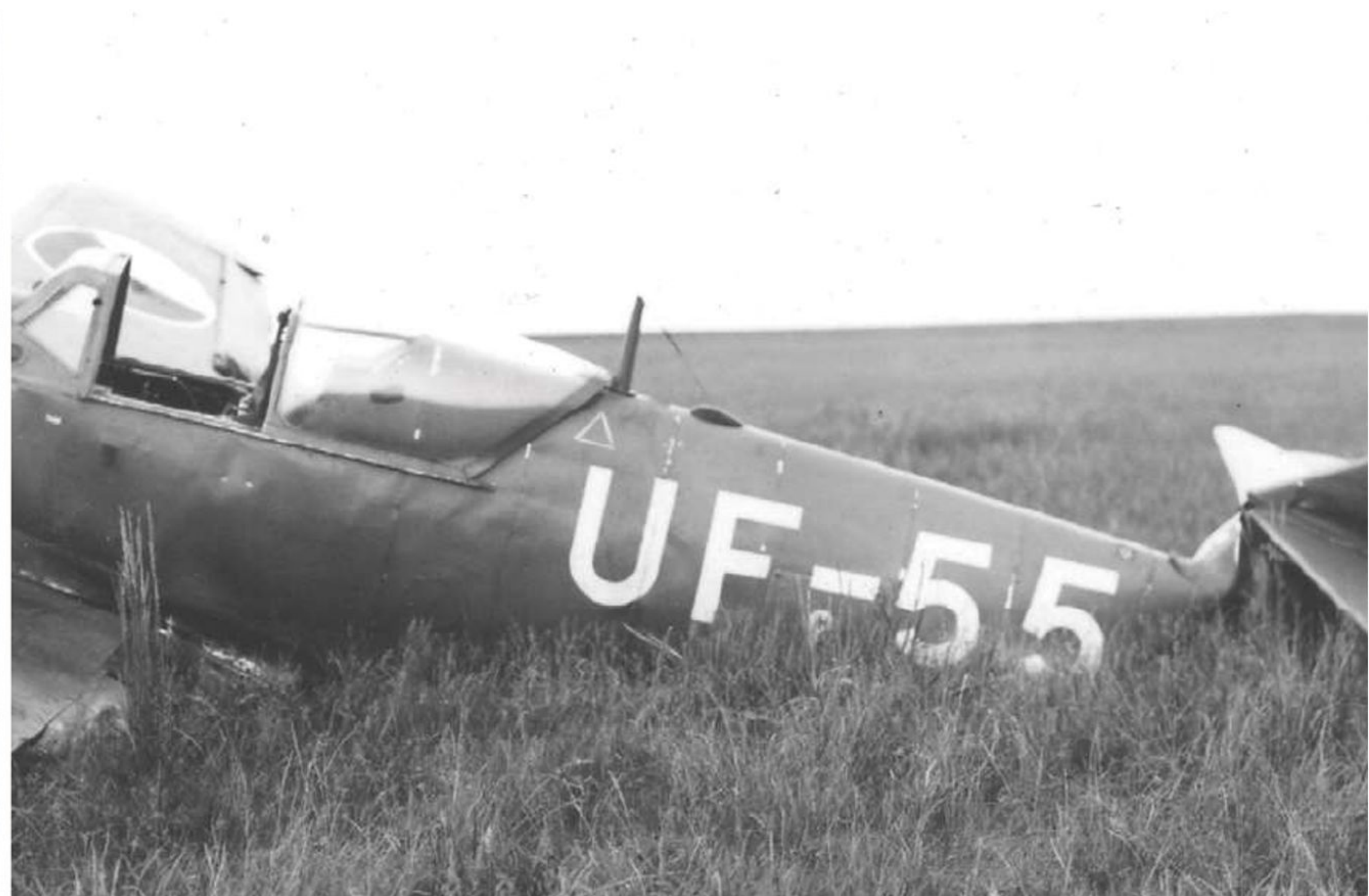
A great example of the fuselage markings painted precisely according to the Attachment No. 2 to the Application and Maintenance of the Marking, order of MNO-VL c. j. 157 Taj. Let. 1946: UF-55 was painted white on the dark base. The aircraft in the photograph, S-199 serial number 543, belonged to the 4th Air Training Squadron and was struck off charge after the crash landing at Prostějov airfield on May 26, 1953.
