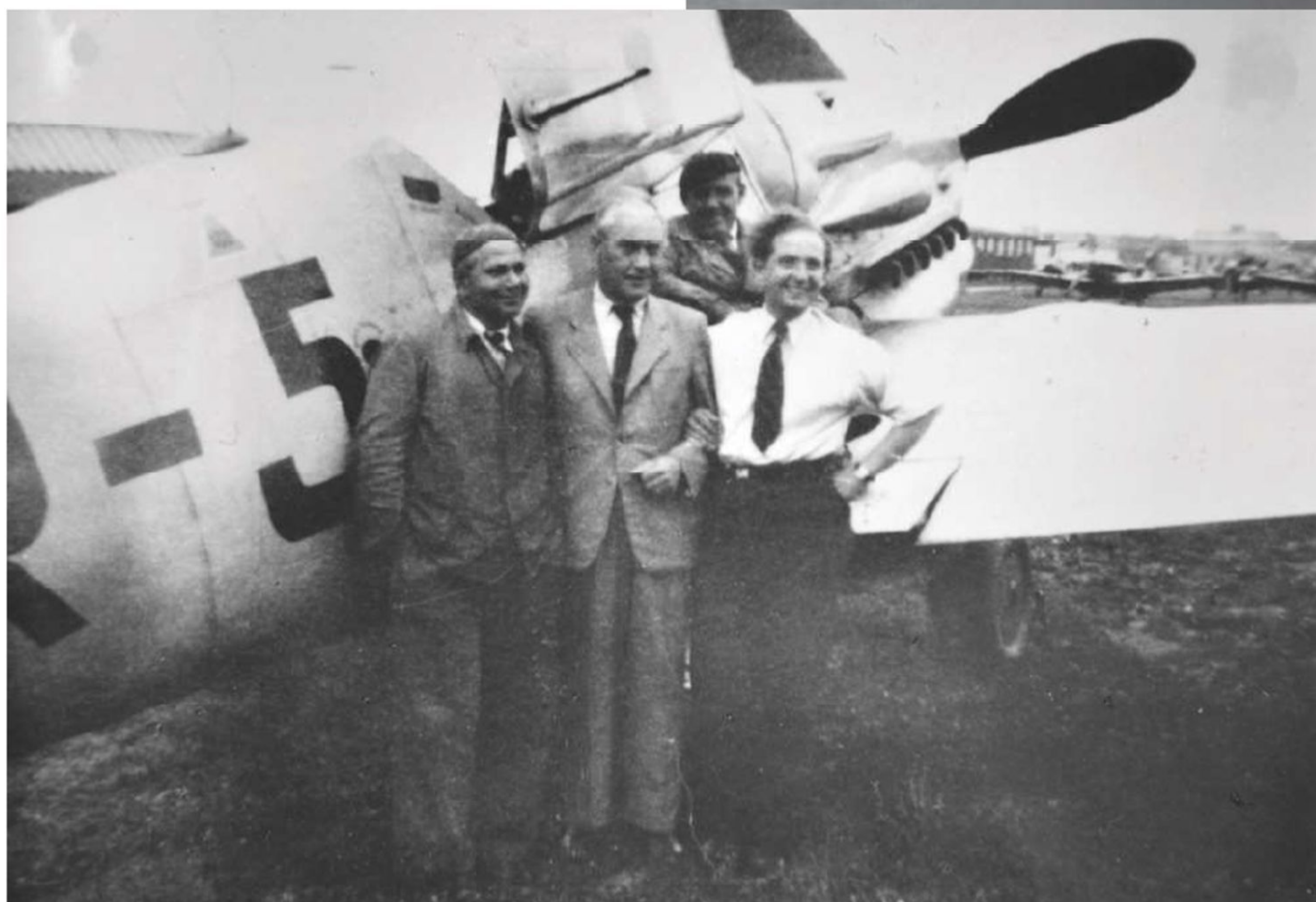
Rather poor quality but interesting photograph captures the aircraft of the staff flight of the 3rd Air Division marked IR-5 with number shaped in an unusual manner. This S-199 could not be identified further but is painted light green-gray overall and features the older type of "Erla Haube" canopy opening to the side.
