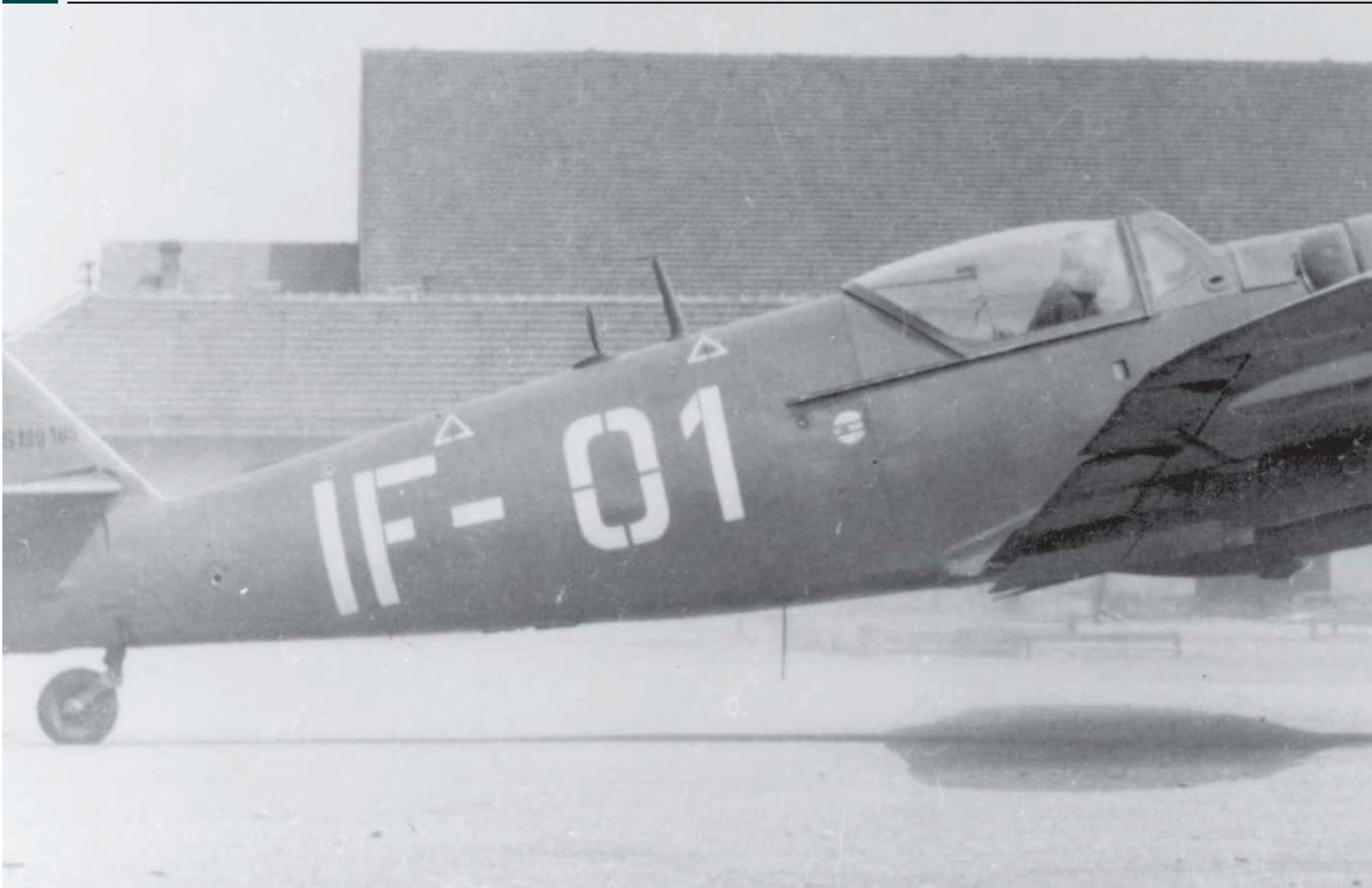
The dark green camouflaged S-199.185 with white code IF-01, originally belonging to 1st Squadron of 51. lp (51st Air Regiment) in Pilsen. There are clear gaps left by "bridges" of the template in the lines of individual letters and numbers.
