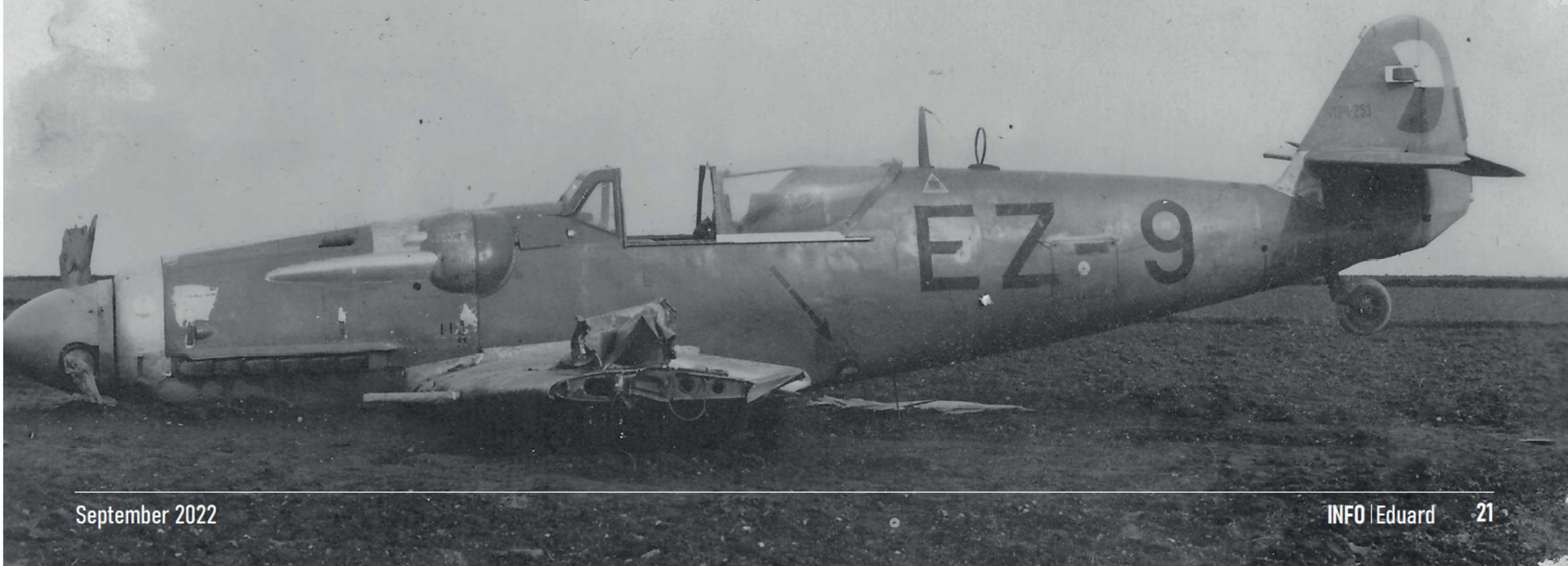
Avia S-199.253, "black" EZ-9 from the 3rd flight of the 5th Fighter Squadron in Plana at Ceske Budejovice as mentioned in this article, demonstrating the attractive camouflage. This emergency landing resulting in the damaged wing and the bottom of the fuselage was performed by WO Jiljí Horak. Notice the unpainted metal skin panels on the nose, cowling and replacement fuselage-vertical tail fairing. The aircraft also features the very thin outline on the vertical tail surfaces national insignia. Of interest are also the protective fabric covers on the fuselage and wing machine guns.
