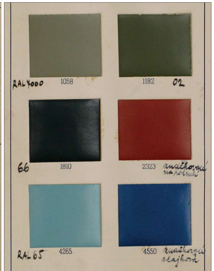
A reproduction of a page from the color chips of shades produced by the National Factory for Paints and Varnishes from 1950, with the original notes preserved. The top row contains samples of light green-grey (RAL equivalents) and Avion 2036.02 (RLM 02), while in the bottom right corner is a shade of blue for that component of the national marking (labeled as Flag) Shade 66 corresponds to RLM 66 Black-Grey (for interiors and wheel wells) and RLM 65 corresponding to shades used on the lower surfaces (Avion 2036.65).
