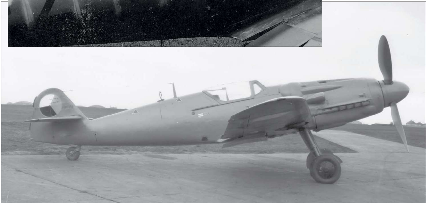
A brand-new Avia S-199, Serial Number 167, made its acceptance flight by Avia's test pilot Antonín Kraus on October 25, 1948. The aircraft is armed with two 17/7 9N wing guns of 7.92mm calibre. Despite the photograph being somewhat underexposed, it is possible to conclude that the scheme is the light green-grey type applied to early aircraft. This aircraft was coded KS-22 and was later attached to the 2nd Flight of the Air Regiment 4 bearing the name of Alois Vašátko, at Plzeň-Skvrňany, where it was damaged in a landing accident on February 11, 1949.
